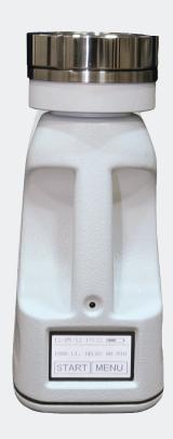
The instrument should be positioned in a spot that is critical for the sterility of the product environment (e.g. near the filling of the final product). On the other hand, if sampling is made during the presence of personnel (e.g. during a surgical operation) the instrument should be positioned in a spot that will not interfere with the activity of the personnel. Consider using a tripod to ensure that the instrument is not knocked over by personnel.
